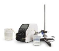
decreases. This is because the laminar flow rate depends on the viscosity, the inside diameter of the hose, and the pressure drop at the ends of the hose. The laminar flow velocity is calculated using Poiseuil's formula: -
